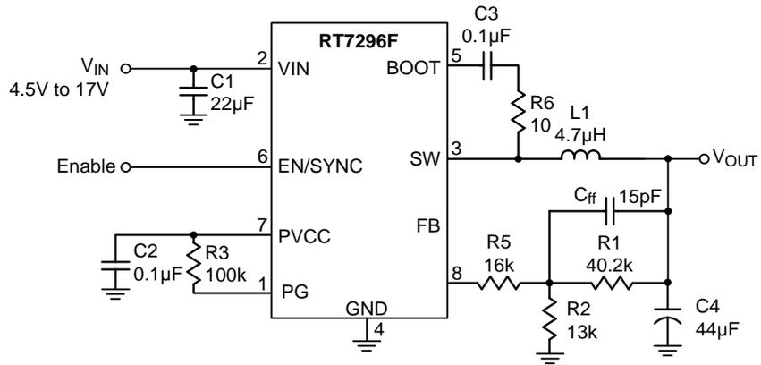
Note : All input and output capacitance in the suggested parameter mean the effective capacitance. The effective capacitance needs to consider any De-rating Effect like DC Bias.
