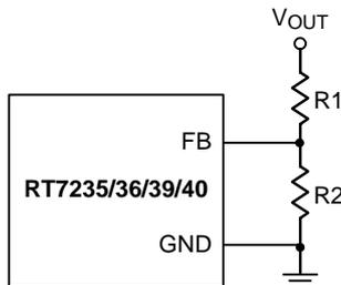
Figure 4. Output Voltage Setting
