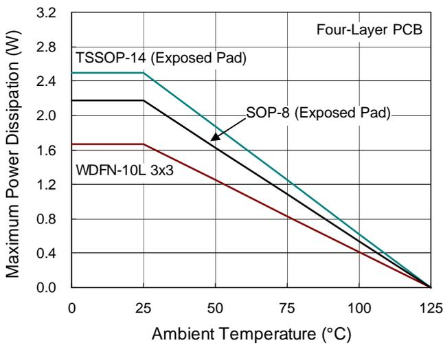
Figure 6. Derating Curve of Maximum Power Dissipation
