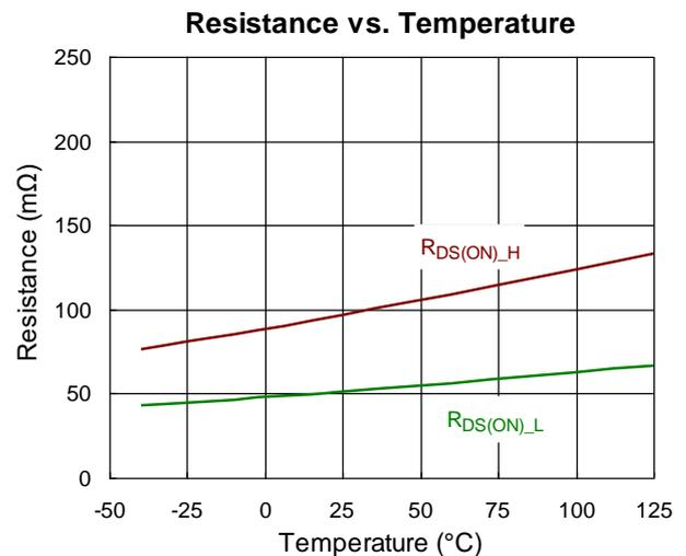
Figure 13. RT6253A/B  $R_{DS(ON)}$  vs. Temperature
