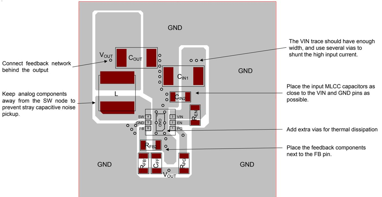
Figure 13. Layout Guide for WDFN-6L 2x2
