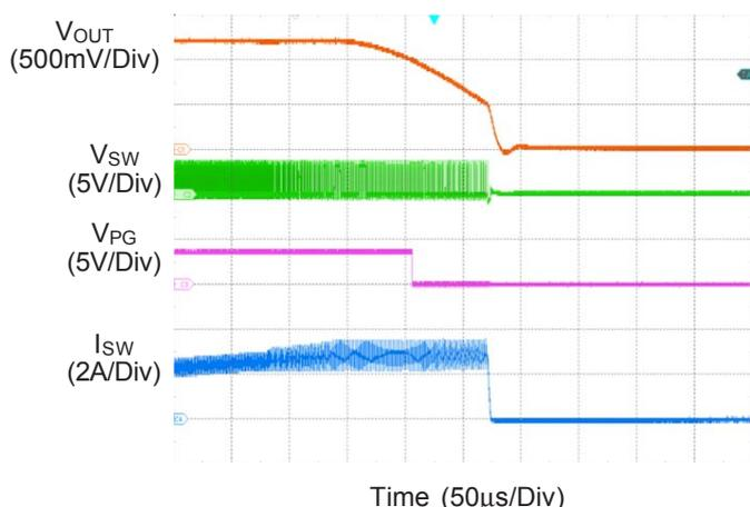
Figure 2. Over-Current Protection
