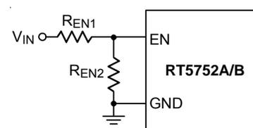
Figure 8. Resistive Divider for Under-Voltage Lockout Threshold Setting
