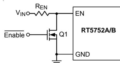
Figure 7. Logic Control for the EN Pin
