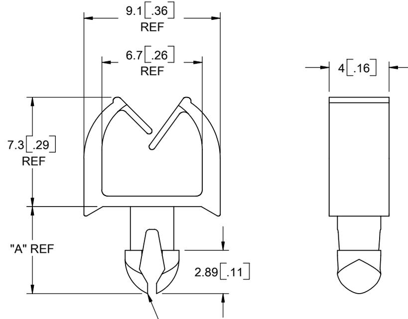
TO SNAP-LOCK IN A 3±0.05 [.118±.002] HOLE DIA.,
