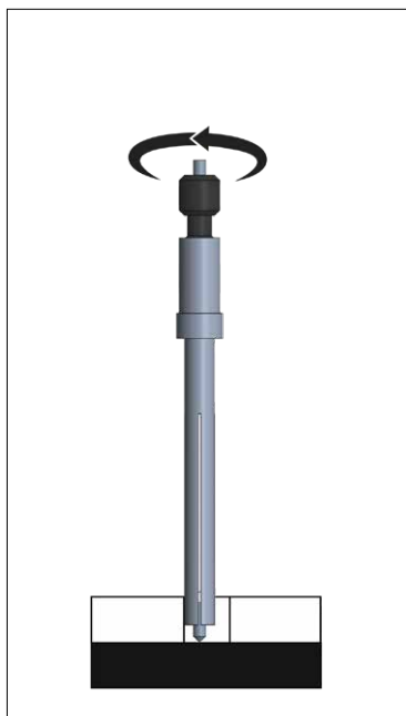
1. Insert centring punch of appropriate size into bore hole, turn the knurled screw
