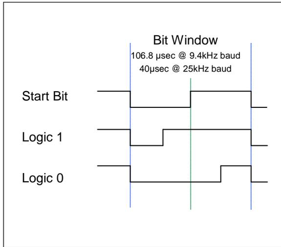
Start bit = 50% duty cycle used to set up strobe time
