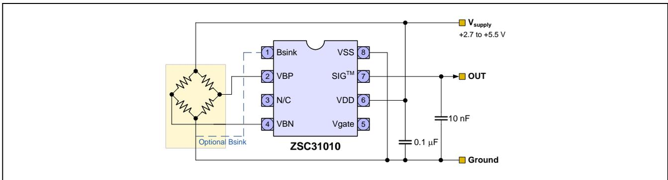
The optional bridge sink allows power savings switching off the bridge current. The output voltage can be one of the following options:
