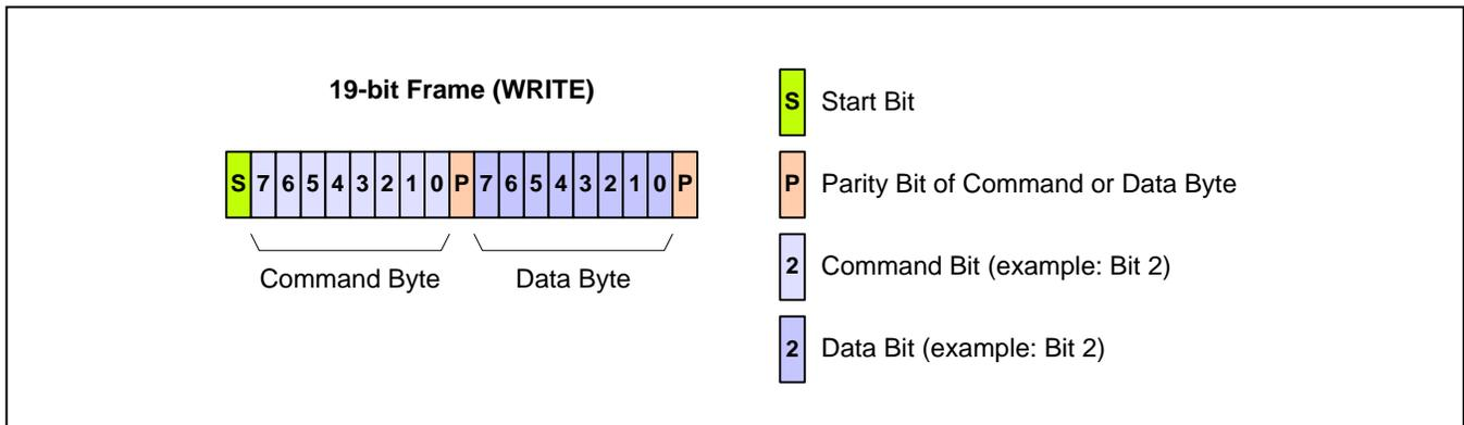
The incoming serial signal will be sampled at a 512 kHz clock rate. This protocol is very tolerant to clock skew and can easily tolerate baud rates in the 6 kHz to 48 kHz range.
