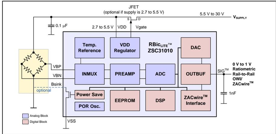
**Rail-to-Rail Ratiometric Voltage Output Applications**
