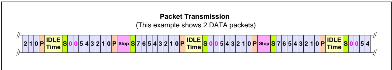
Table 3.2 shows the idle time between packets versus the update rate. This idle time can vary by nominal +/-15% between parts, and over a temperature range of -50 to 150°C.
