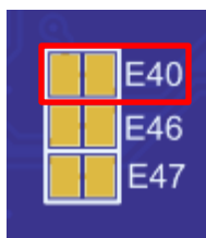
Figure 20. Jumper for User Switch (S1) (Bottom view)
