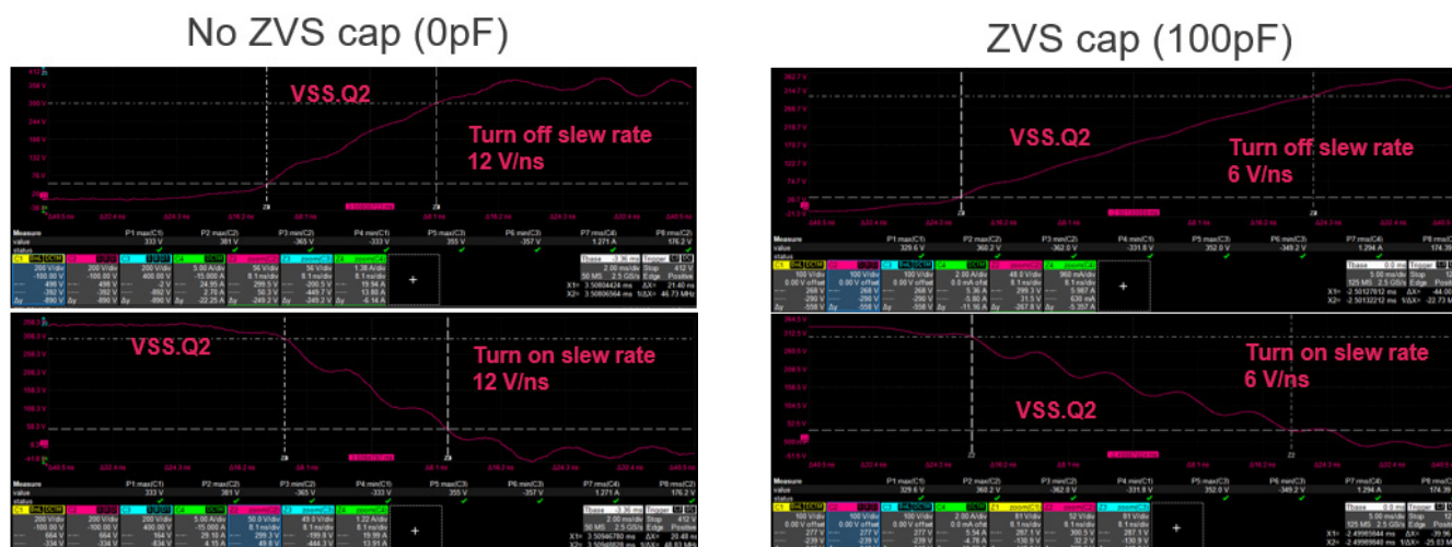
Figure 16. ZVS Capacitor Slew Rate Control
