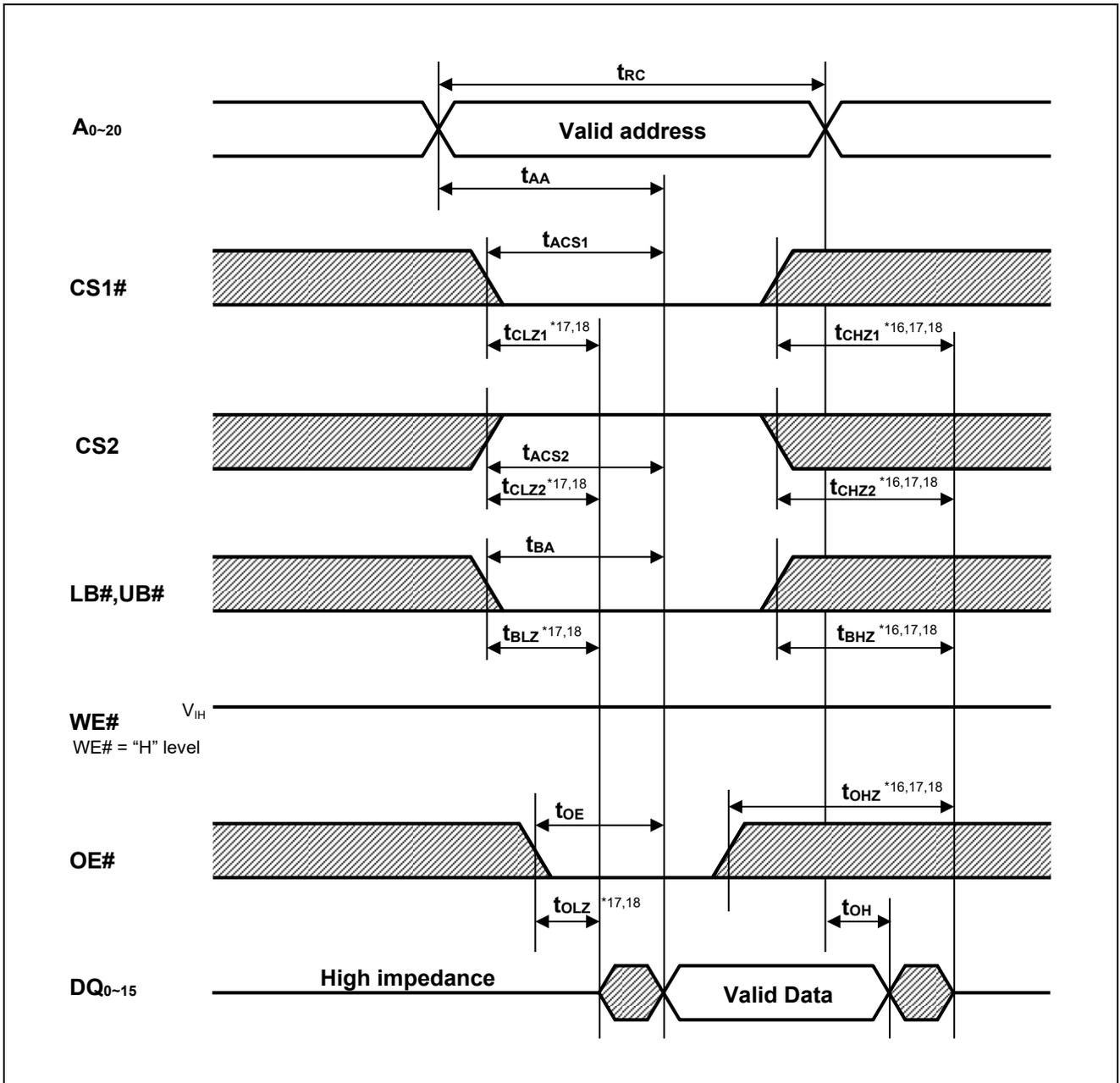
Note 16.  $t_{CHZ1}$ ,  $t_{CHZ2}$ ,  $t_{BHZ}$  and  $t_{OHZ}$  are defined as the time when the DQ pins enter a high-impedance state and are not referred to the DQ levels.
