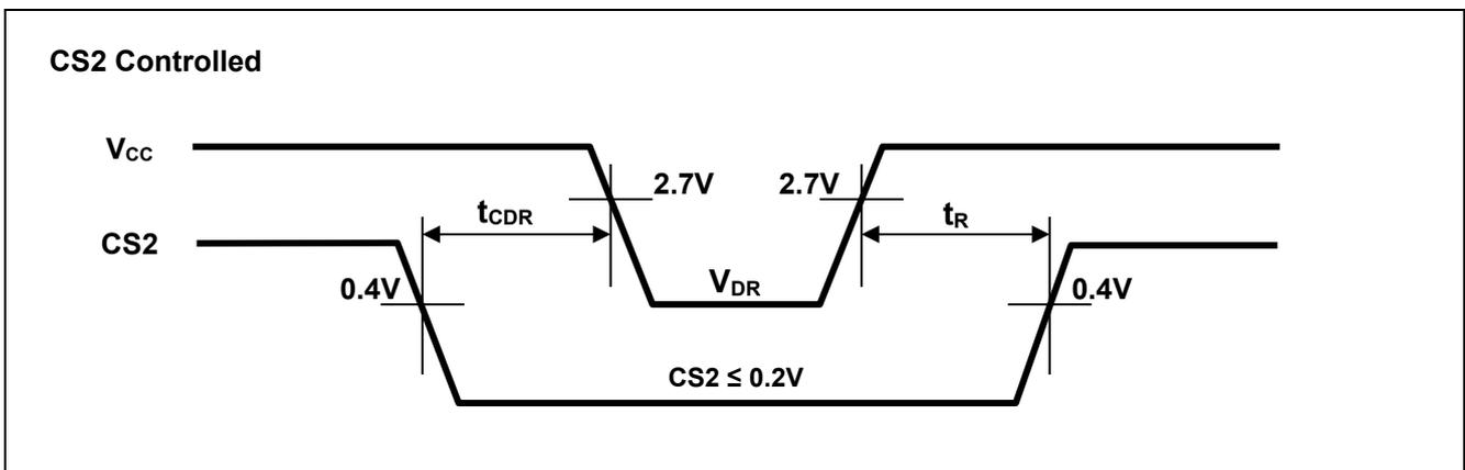
Low Vcc Data Retention Timing Waveforms (LB#,UB# controlled)
