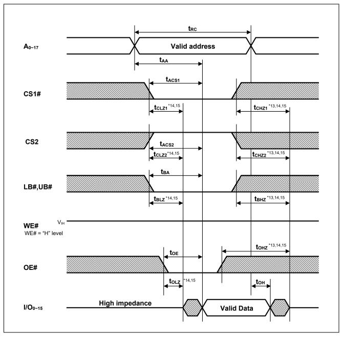
Note 13. t<sub>CHZ1</sub>, t<sub>CHZ2</sub>, t<sub>BHZ</sub> and t<sub>OHZ</sub> are defined as the time when the I/O pins enter a high-impedance state and are not referred to the I/O levels.
