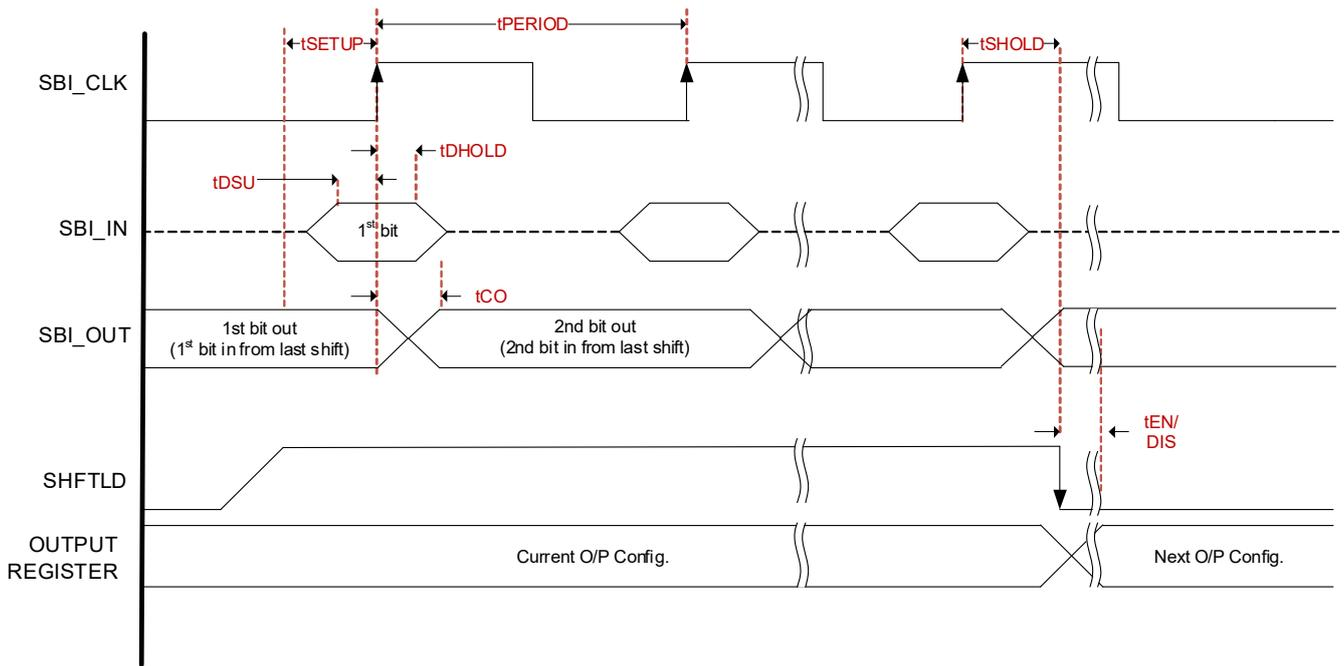
Figure 10. Side-Band Interface Timing
