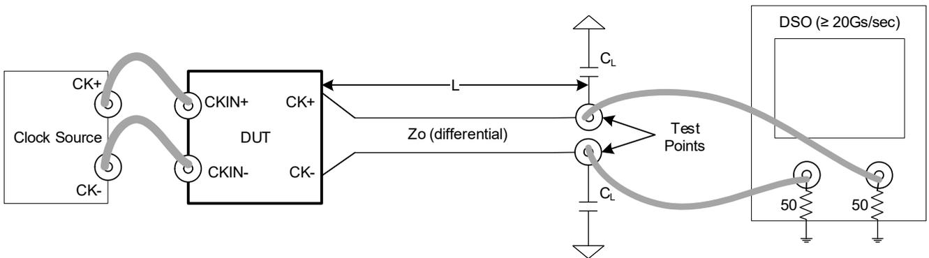
Figure 12. AC/DC Test Load for Differential Outputs (Double-Terminated)
