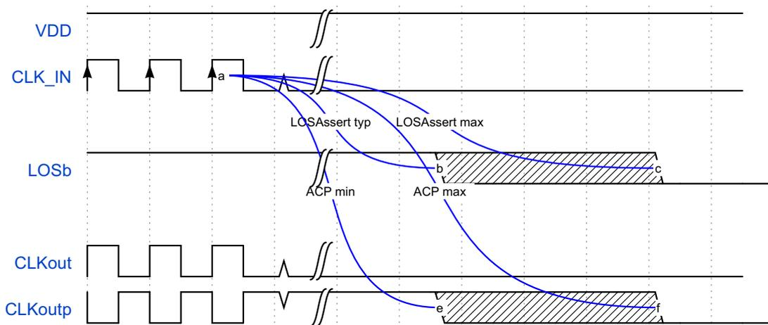
Figure 23. LOSb Assert Timing
