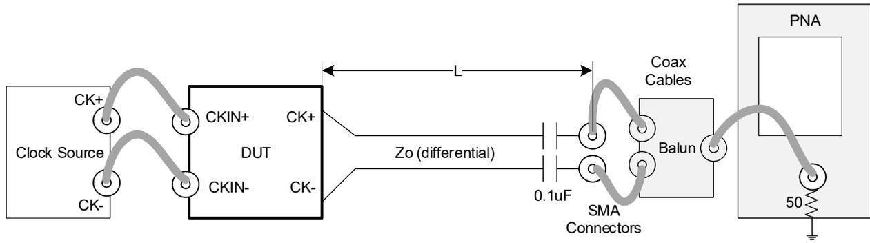
Figure 13. Test Load for PCIe Phase Jitter Measurements
