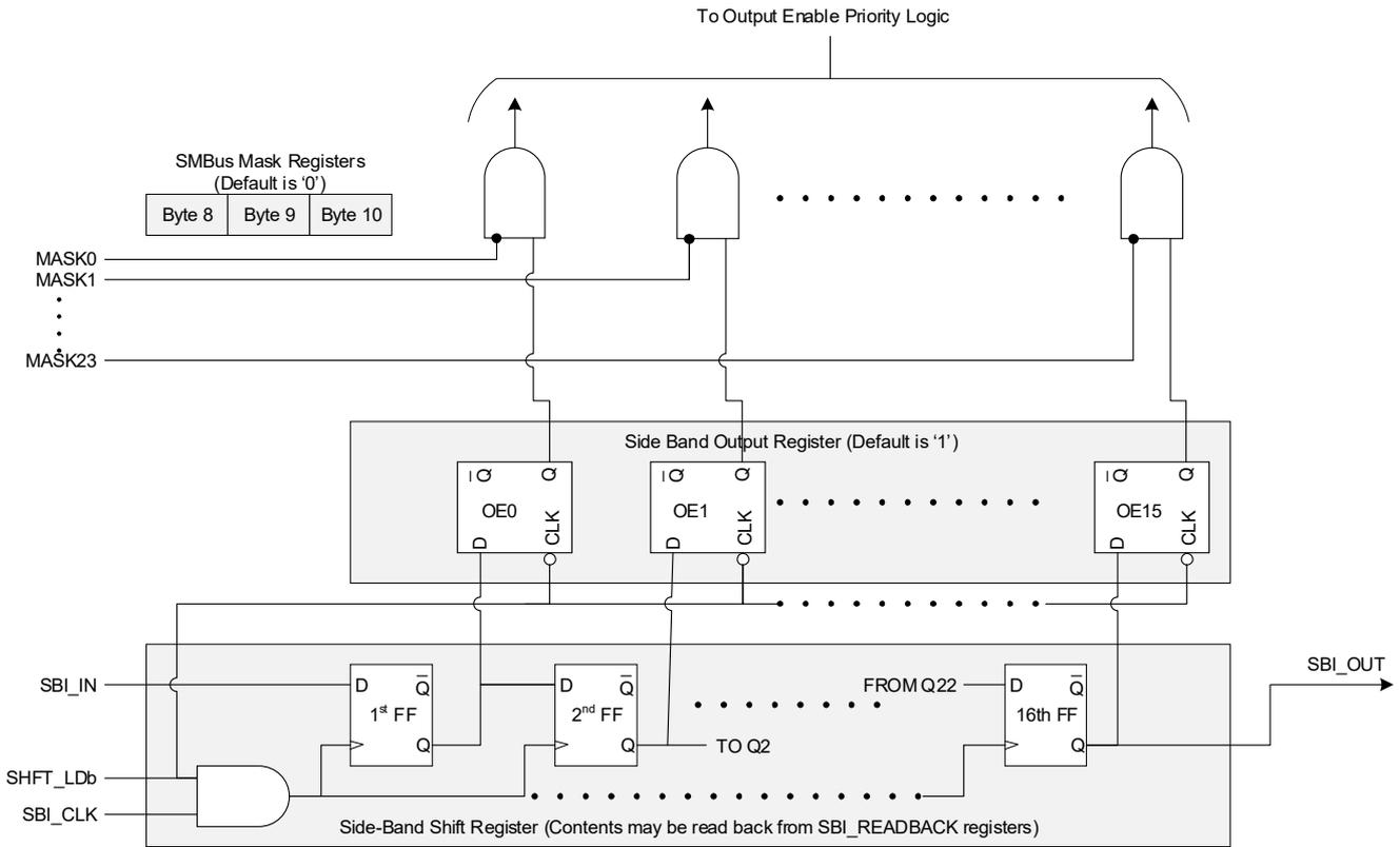
Figure 24. Side-band Interface High-Level Functional Diagram (RC192xx shown)
