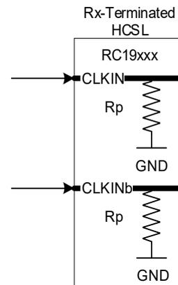
Figure 17. Receiver Termination
