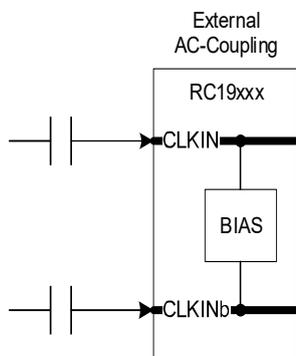
Figure 16. External AC-Coupling
