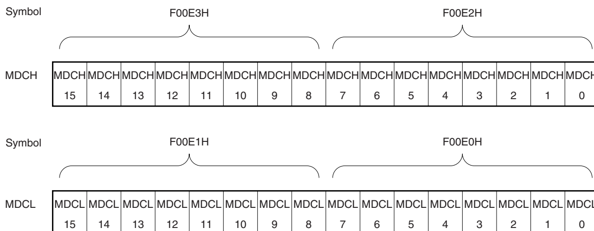
Figure 18-4. Format of Multiplication/Division Data Register C (MDCH, MDCL)
