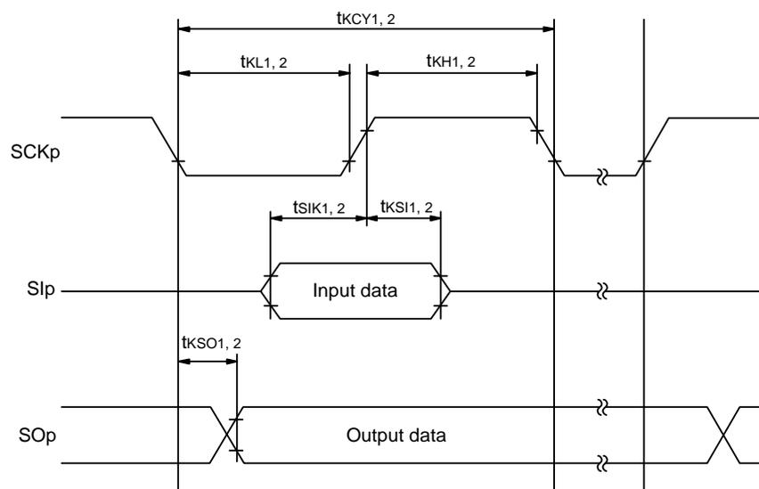
**CSI mode serial transfer timing (during communication at same potential)
