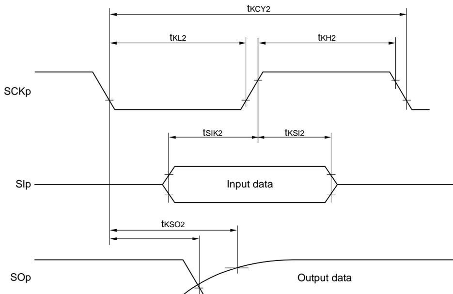
**CSI mode serial transfer timing (slave mode) (during communication at different potential)
