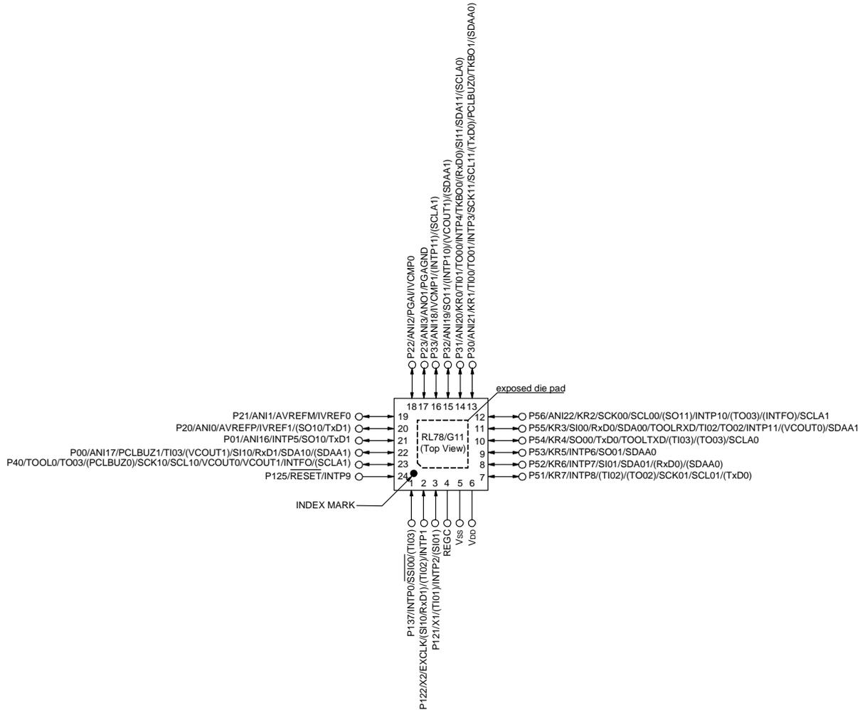
**Caution** Connect the REGC pin to Vss pin via a capacitor (0.47 to 1 μF).
