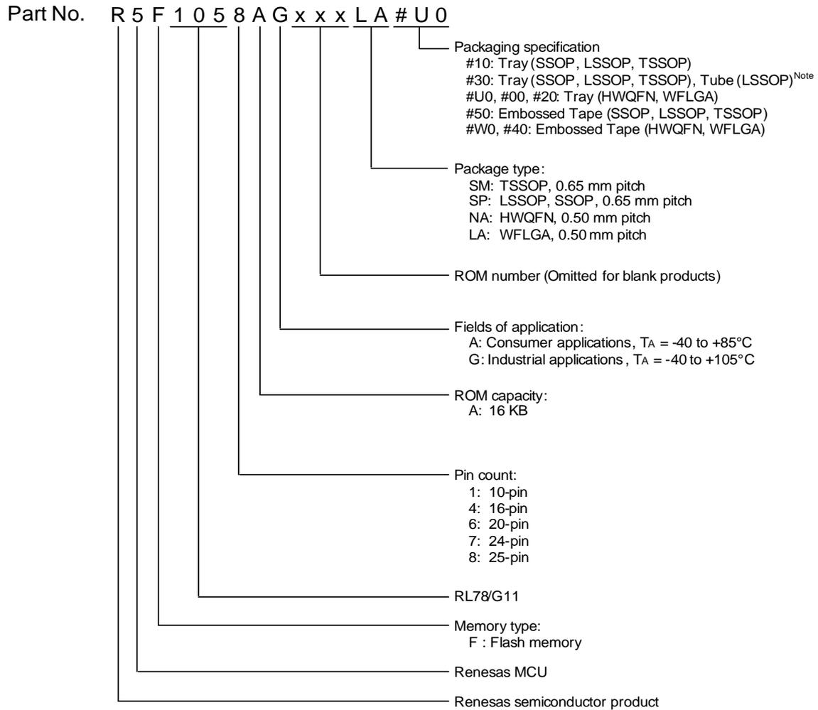
**Note** The packaging specification is only "Tube" for products in the 20-pin LSSOP.
