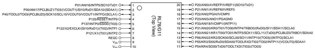
**Caution** Connect the REGC pin to Vss pin via a capacitor (0.47 to 1 μF).
