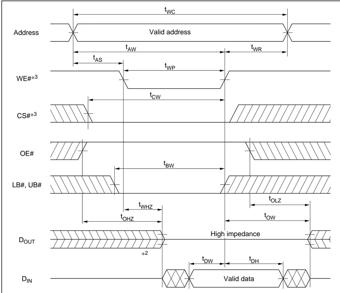
Write Timing Waveform (2) (CS# Controlled)
