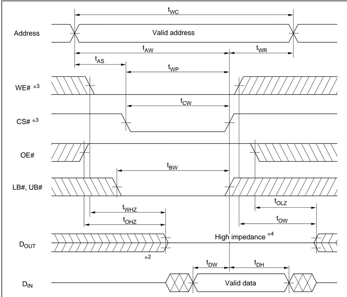
Write Timing Waveform (3) (LB#, UB# Controlled, OE# = V<sub>ih</sub>)
