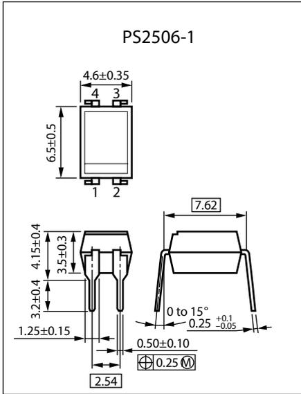
**Lead Bending Type For Surface Mount**
