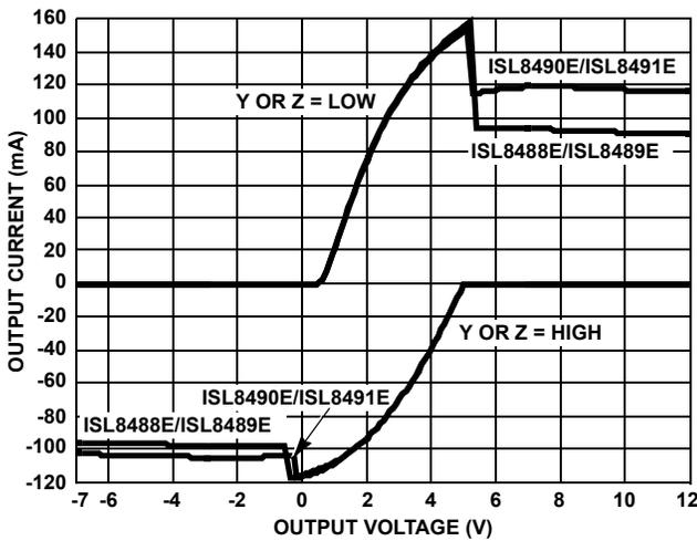
FIGURE 8. DRIVER OUTPUT CURRENT vs SHORT CIRCUIT VOLTAGE
