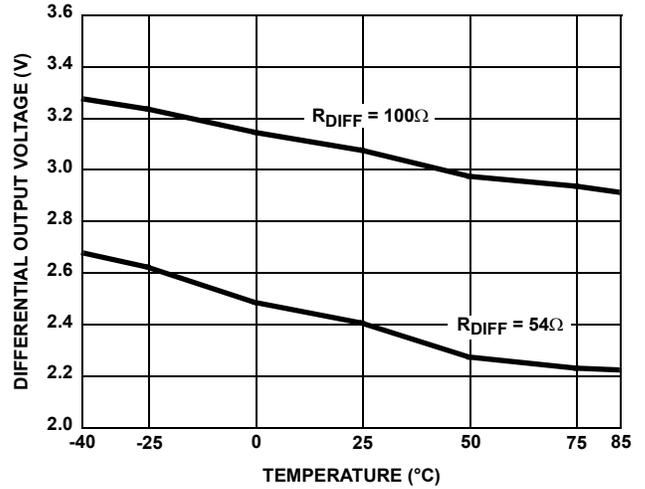
FIGURE 7. DRIVER DIFFERENTIAL OUTPUT VOLTAGE vs TEMPERATURE
