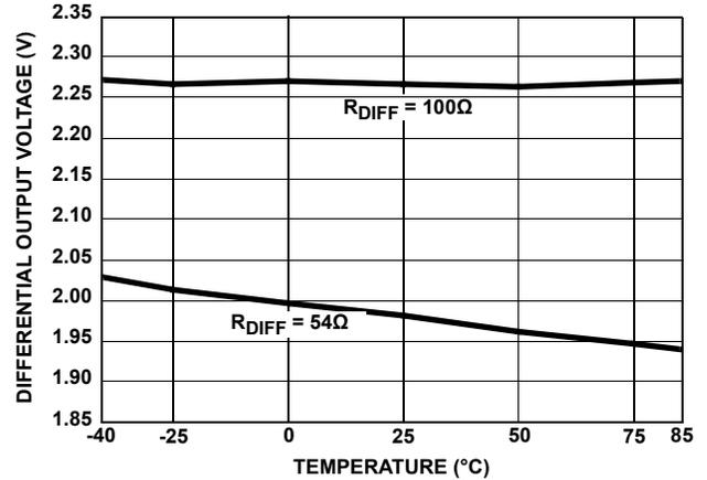
FIGURE 8. DRIVER DIFFERENTIAL OUTPUT VOLTAGE vs TEMPERATURE
