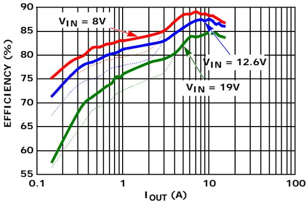
FIGURE 34. 1-PHASE DEM EFFICIENCY, VID = 0.875V, DPRSLPVR IS ASSERTED FOR I<sub>OUT</sub> < 3A V<sub>IN1</sub> = 8V, V<sub>IN2</sub> = 12.6V AND V<sub>IN3</sub> = 19V. SOLID LINES: ISL62882C EFFICIENCY, DOTTED LINES: WOULD-BE EFFICIENCY IF LGATE1b WAS NOT TURNED OFF IN DPRSLPVR MODE
