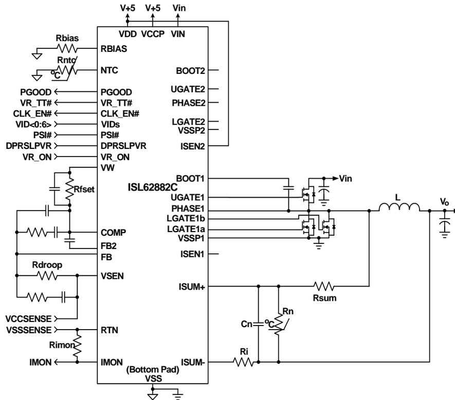
FIGURE 3. TYPICAL 1-PHASE APPLICATION CIRCUIT USING DCR SENSING
