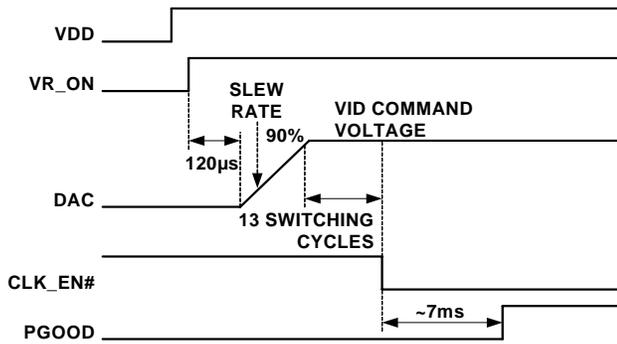
FIGURE 11. SOFT-START WAVEFORMS FOR GPU VR APPLICATION
