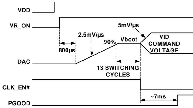
FIGURE 10. SOFT-START WAVEFORMS FOR CPU VR APPLICATION
