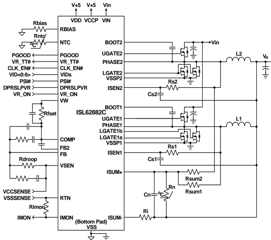
FIGURE 1. TYPICAL 2-PHASE APPLICATION CIRCUIT USING DCR SENSING
