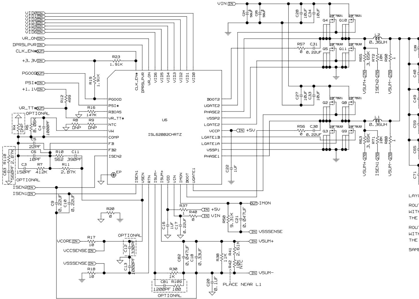
FIGURE 31. 2-PHASE CPU APPLICATION REFERENCE DESIGN
