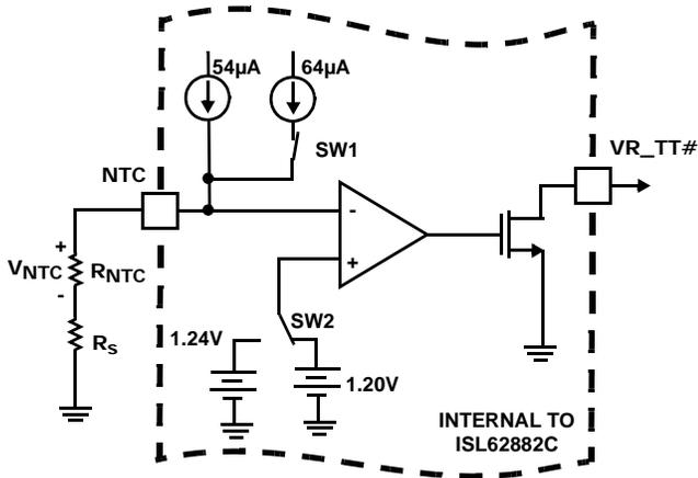
FIGURE 29. CIRCUITRY ASSOCIATED WITH THE THERMAL THROTTLING FEATURE
