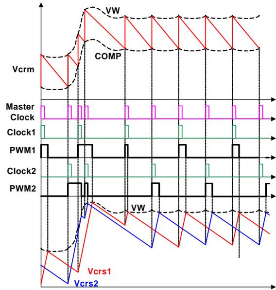
FIGURE 7. R<sup>3</sup>™ MODULATOR OPERATION PRINCIPLES IN LOAD INSERTION RESPONSE
