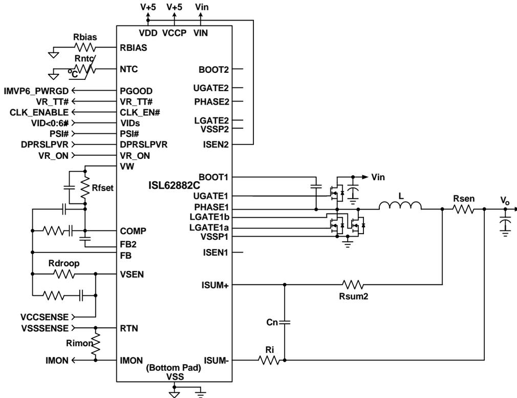
FIGURE 4. TYPICAL 1-PHASE APPLICATION CIRCUIT USING RESISTOR SENSING
