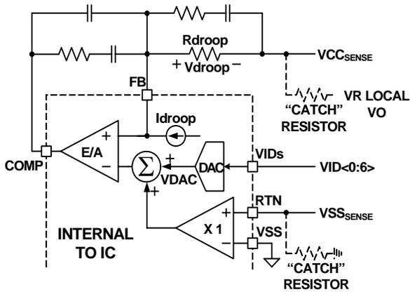
**FIGURE 12. DIFFERENTIAL SENSING AND LOAD LINE IMPLEMENTATION**
