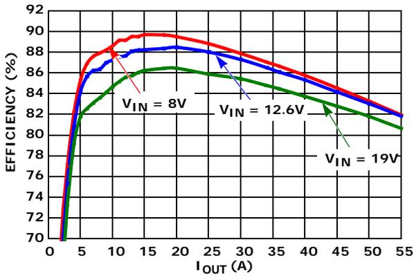
FIGURE 32. 2-PHASE CCM EFFICIENCY, VID = 1.075V, V<sub>IN1</sub> = 8V, V<sub>IN2</sub> = 12.6V AND V<sub>IN3</sub> = 19V
