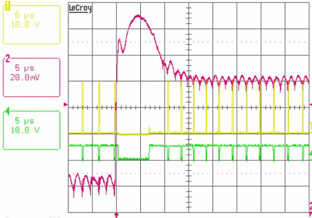
FIGURE 50. TRANSIENT RESPONSE WITH OVERSHOOT REDUCTION FUNCTION ENABLED,  $V_{IN} = 19V$ ,  $V_{ID} = 0.95V$ ,  $I_O = 12A/51A$ ,  $di/dt = \text{“FASTEST”}$ , Ch1: PHASE1, Ch2:  $V_O$ , Ch3: N/A, Ch4: LGATE1
