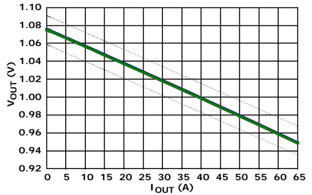
FIGURE 33. 2-PHASE CCM LOAD LINE, VID = 1.075V, V<sub>IN1</sub> = 8V, V<sub>IN2</sub> = 12.6V AND V<sub>IN3</sub> = 19V
