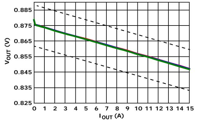
FIGURE 35. 1-PHASE DEM LOAD LINE, VID = 0.875V, DPRSLPVR IS ASSERTED FOR I<sub>OUT</sub> < 3A V<sub>IN1</sub> = 8V, V<sub>IN2</sub> = 12.6V AND V<sub>IN3</sub> = 19V.
