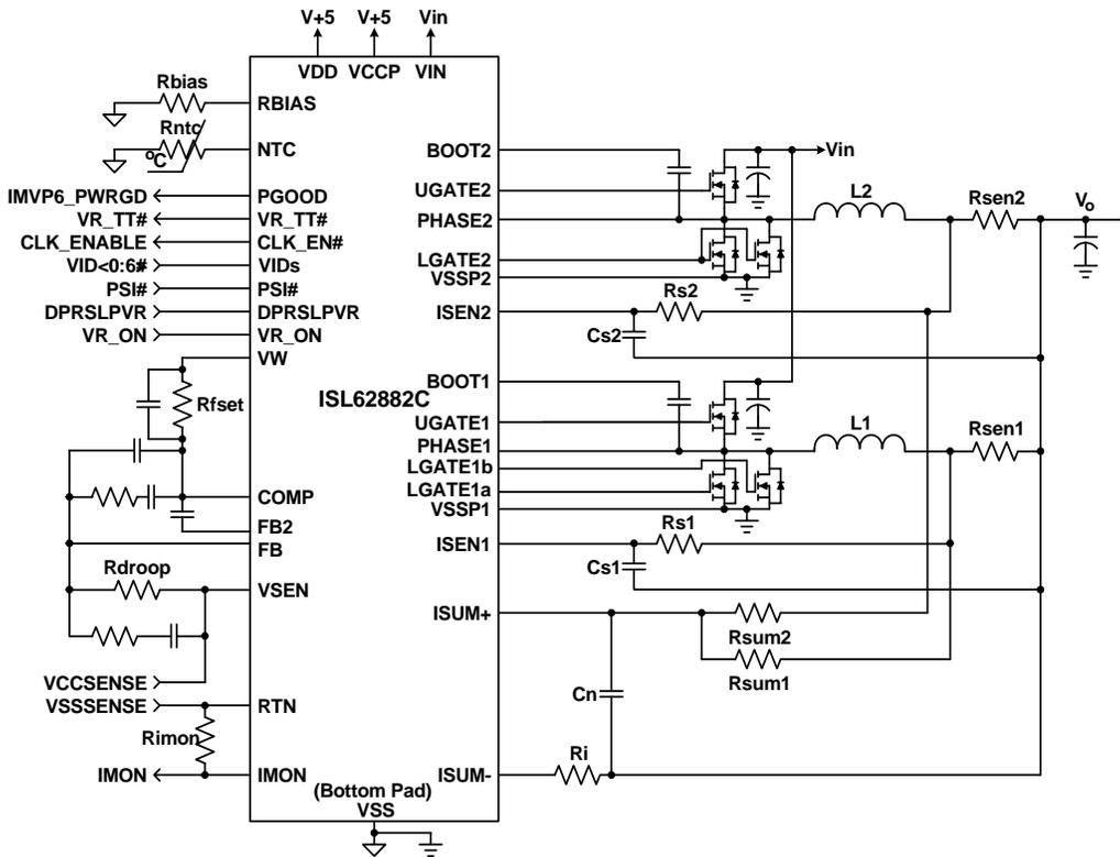
FIGURE 2. TYPICAL 2-PHASE APPLICATION CIRCUIT USING RESISTOR SENSING
