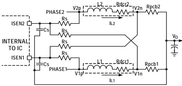
**FIGURE 14. DIFFERENTIAL-SENSING CURRENT BALANCING CIRCUIT**
