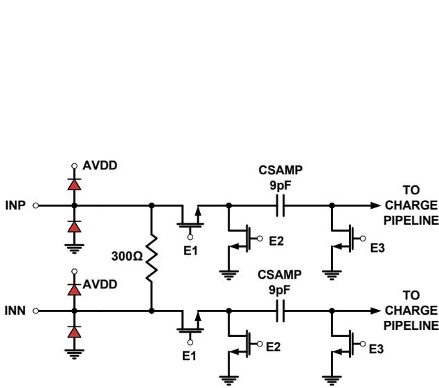
FIGURE 43. ANALOG INPUTS
