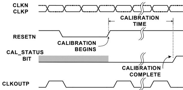
FIGURE 23. CALIBRATION TIMING
