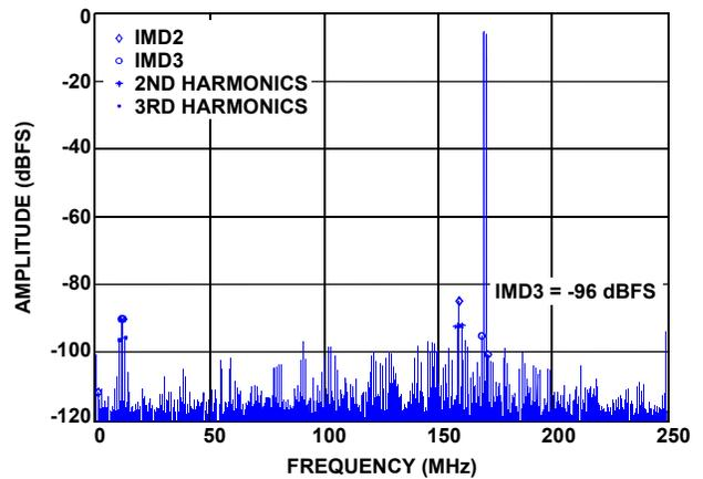
FIGURE 17. TWO-TONE SPECTRUM (F1 = 170MHz, F2 = 171MHz -7dBFS)
