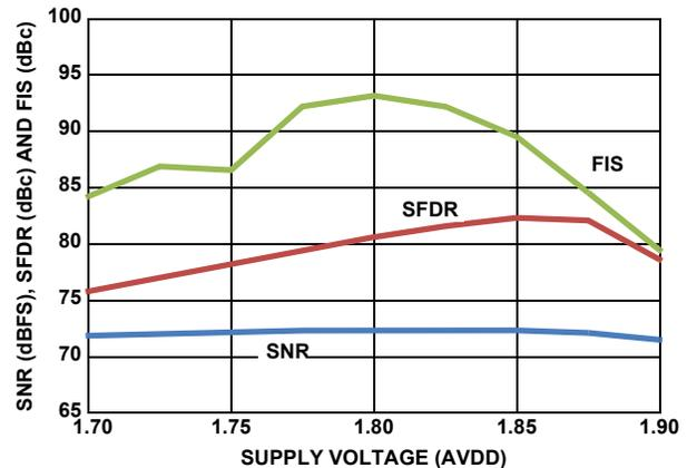
FIGURE 21. ANALOG SUPPLY VOLTAGE SWEEP WITH I2E FROZEN, I2E PREVIOUSLY CALIBRATED AT 1.8V, F<sub>IN</sub> = 105MHz
