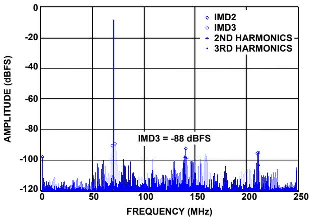
FIGURE 16. TWO-TONE SPECTRUM (F1 = 70MHz, F2 = 71MHz -7dBFS)
