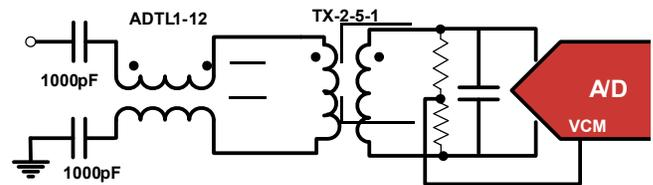
FIGURE 29. TRANSMISSION-LINE TRANSFORMER INPUT FOR HIGH IF APPLICATIONS
