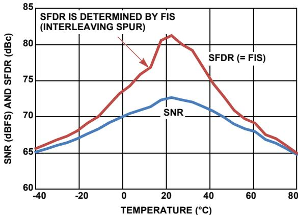
FIGURE 20. TEMPERATURE SWEEP WITH I2E FROZEN, I2E PREVIOUSLY CALIBRATED AT +25 °C, F<sub>IN</sub> = 105MHz
