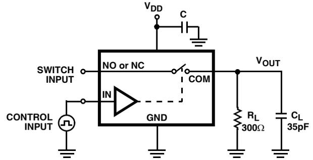
Repeat test for all switches. C<sub>L</sub> includes fixture and stray capacitance.
