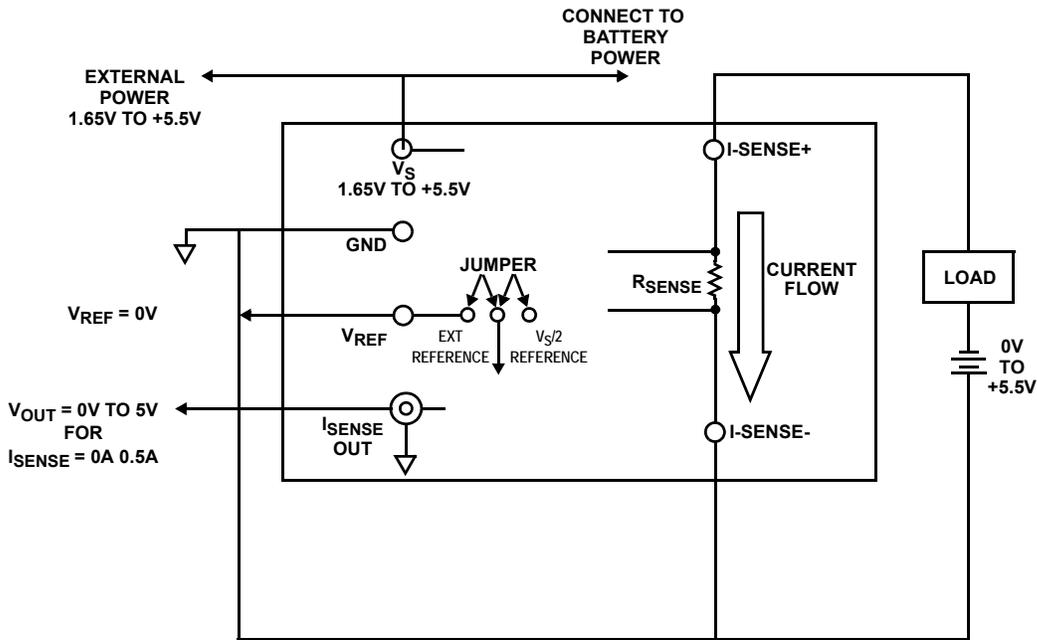
FIGURE 3. CURRENT SENSE FOR LOW SIDE UNI-DIRECTIONAL MEASUREMENT
