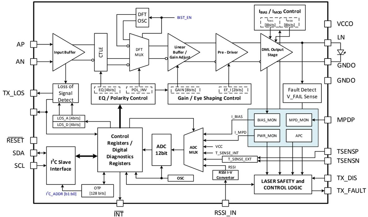
Figure 1: Functional Block Diagram of a Single Channel
