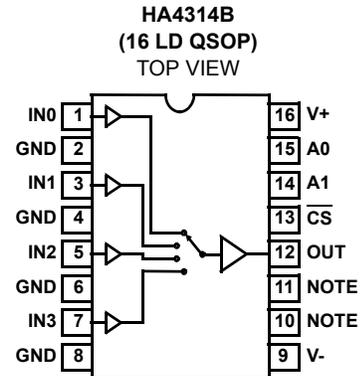
NOTE: These pins must be left floating or connected to ground
