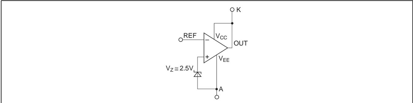
Figure 1 Operation Diagram
