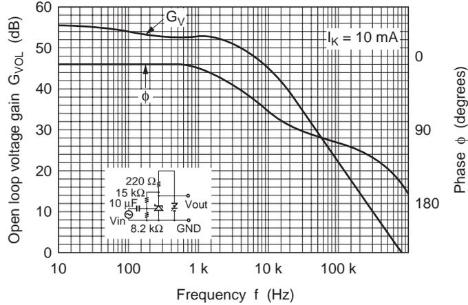
Open Loop Voltage Gain, Phase vs. Frequency Characteristics (2)
