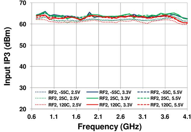
**Input IP3 RF2 Port [T<sub>c</sub> operating = -40C to 105C]**
