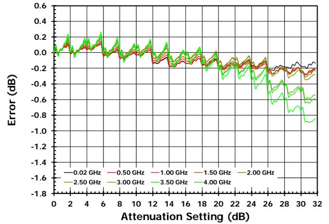
Figure 12. Worst Case Absolute Accuracy vs Frequency [LSB = 0.50dB]
