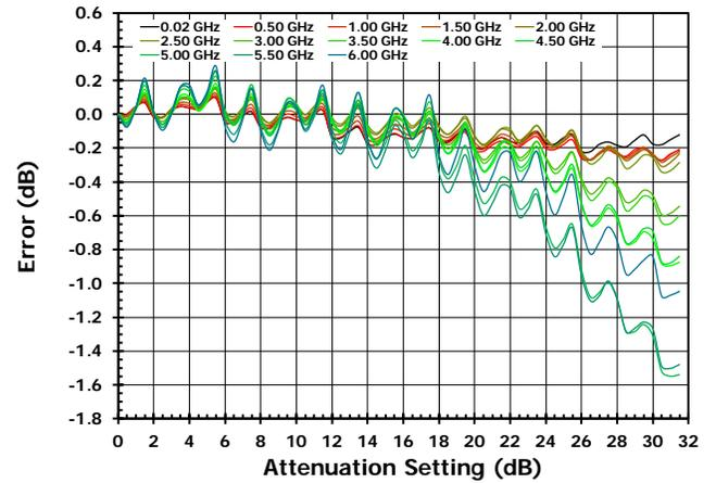
Figure 14. Worst Case Absolute Accuracy vs Frequency [LSB = 1.00dB]
