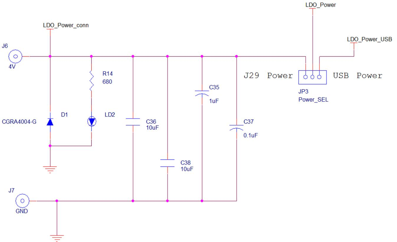
Figure 7. LDO Power Schematic
