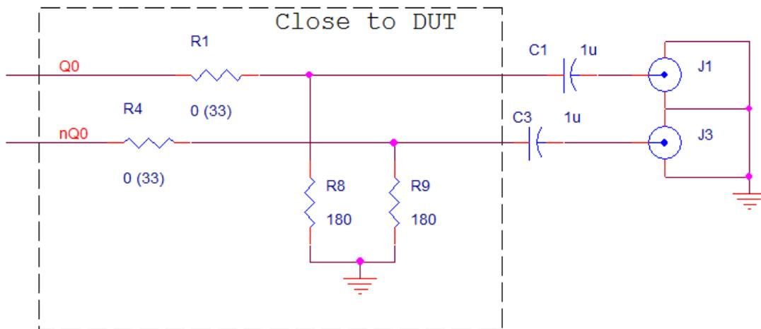
\* If the output frequency is below 50MHz, increase the value of C1 and C3.
