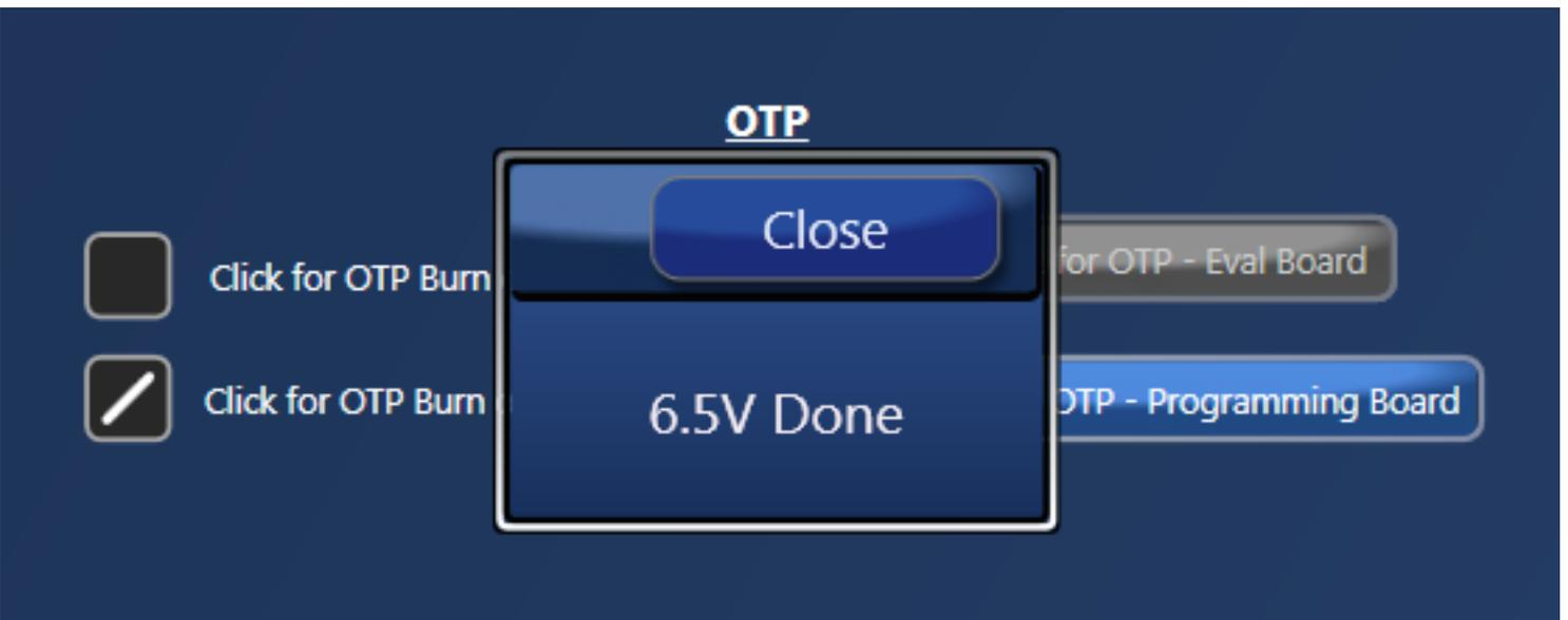
Step 3. Once the previous step is completed, a new window will pop-up confirming to proceed with the OTP burn. Please note that this process cannot be reverted back.
