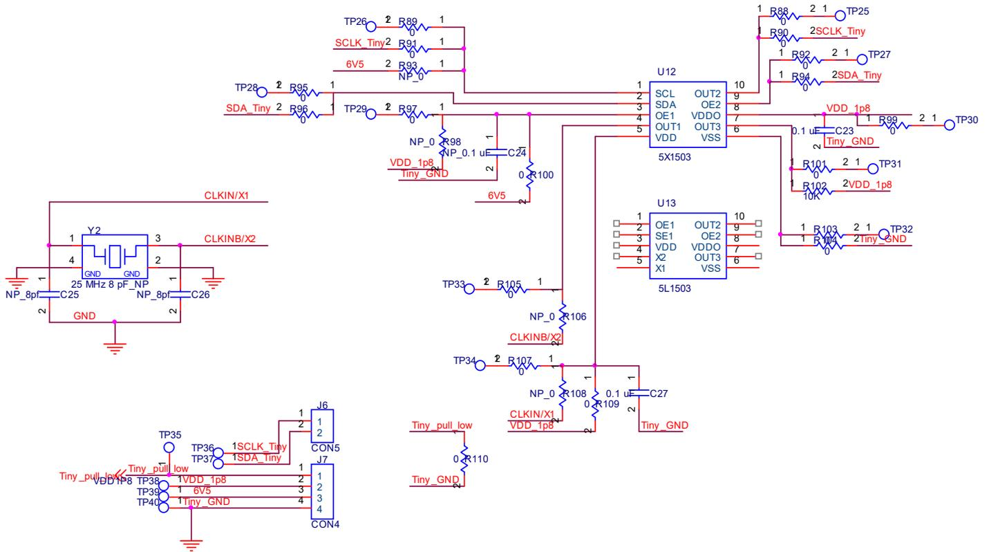
Figure 6. 5X1503 Evaluation Board (board without a crystal)
