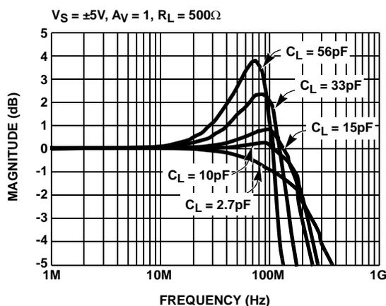
FIGURE 5. FREQUENCY RESPONSE vs C<sub>L</sub>
