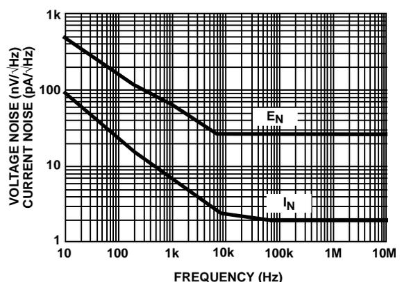
FIGURE 12. VOLTAGE AND CURRENT NOISE vs FREQUENCY
