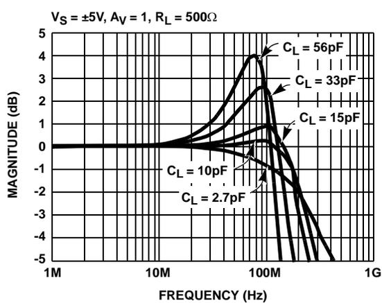
FIGURE 4. FREQUENCY RESPONSE vs C<sub>L</sub>
