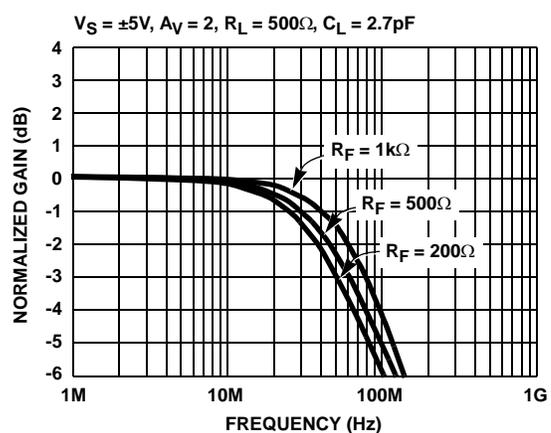
FIGURE 6. FREQUENCY RESPONSE FOR VARIOUS R<sub>F</sub>
