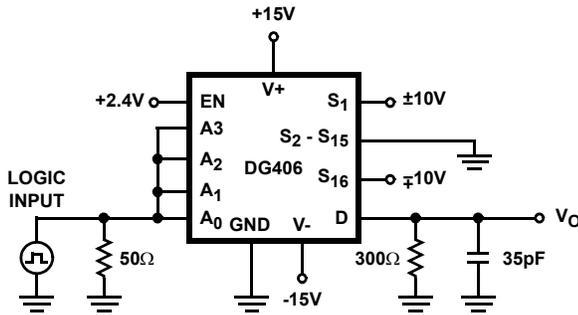
FIGURE 3A. DG406 TEST CIRCUIT
