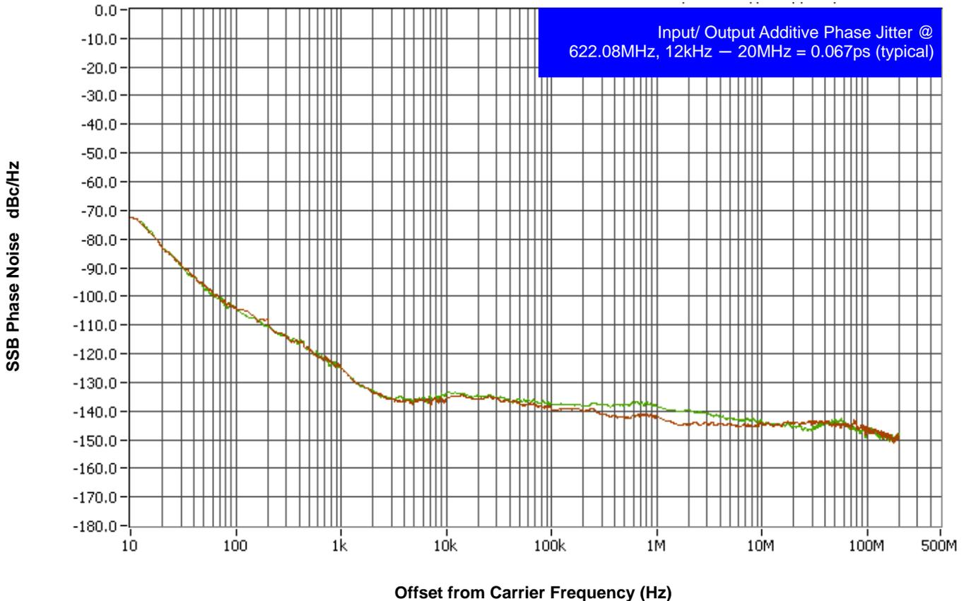
As with most timing specifications, phase noise measurements have issues relating to the limitations of the equipment. Often the noise floor of the equipment is higher than the noise floor of the device. This is illustrated above. The device meets the noise floor of what is shown, but can actually be lower. The phase noise is dependent on the input source and measurement equipment.
