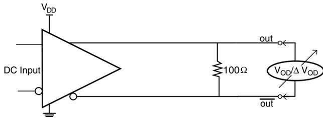
Figure 11. Offset Voltage Setup
