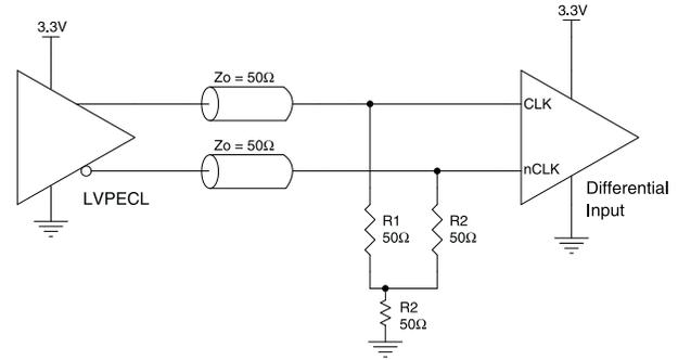
Figure 15. CLK/ nCLK Input Driven by a 3.3V LVPECL Driver
