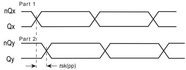
Figure 10. Differential Output Voltage Setup
