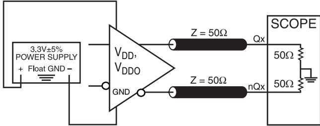
Figure 3. 2.5V Core/ 2.5V Output Load AC Test Circuit
