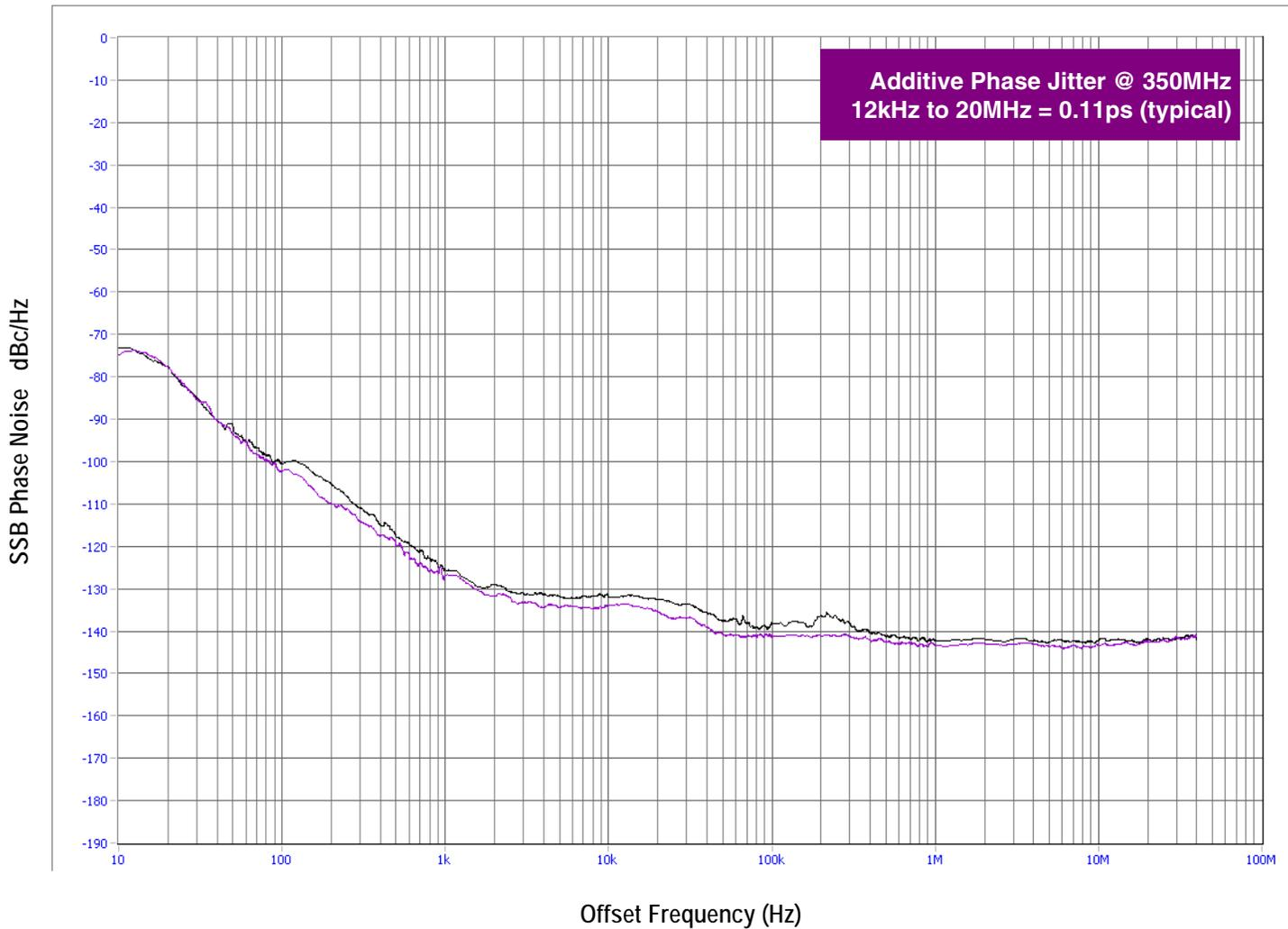
As with most timing specifications, phase noise measurements has issues relating to the limitations of the equipment. Often the noise floor of the equipment is higher than the noise floor of the device.
