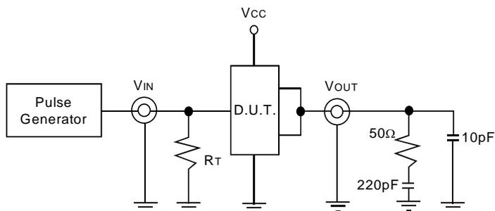
Figure 2.  $Z_o = 50\Omega$  AC Termination,  $C_L = 10pF$
