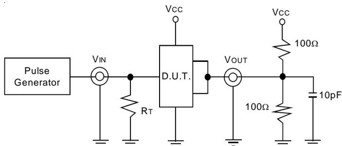
Figure 1.  $Z_o = 50\Omega$  to  $V_{cc}/2$ ,  $C_L = 10pF$
