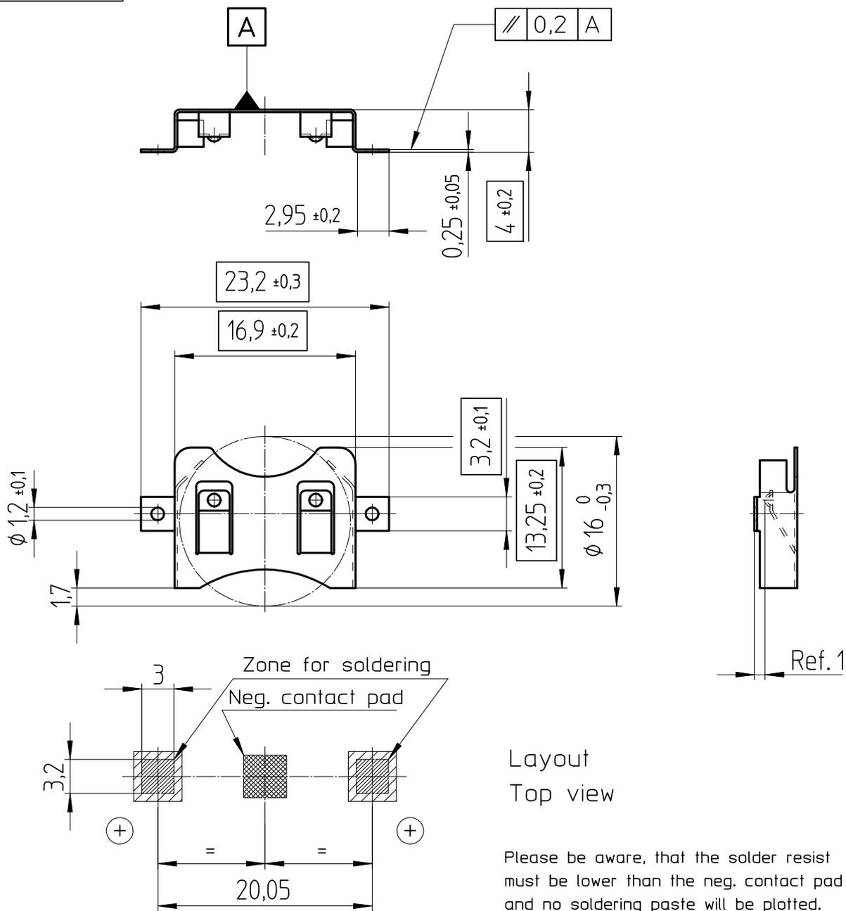
Please be aware, that the solder resist must be lower than the neg. contact pad and no soldering paste will be plotted.
