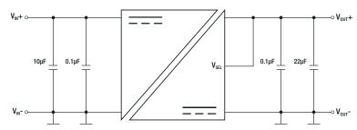
$V_{IN}$ = 3-3.6VDC,  $V_{OUT}$ = 3.3VDC,  $I_{OUT}$ = 200mA
