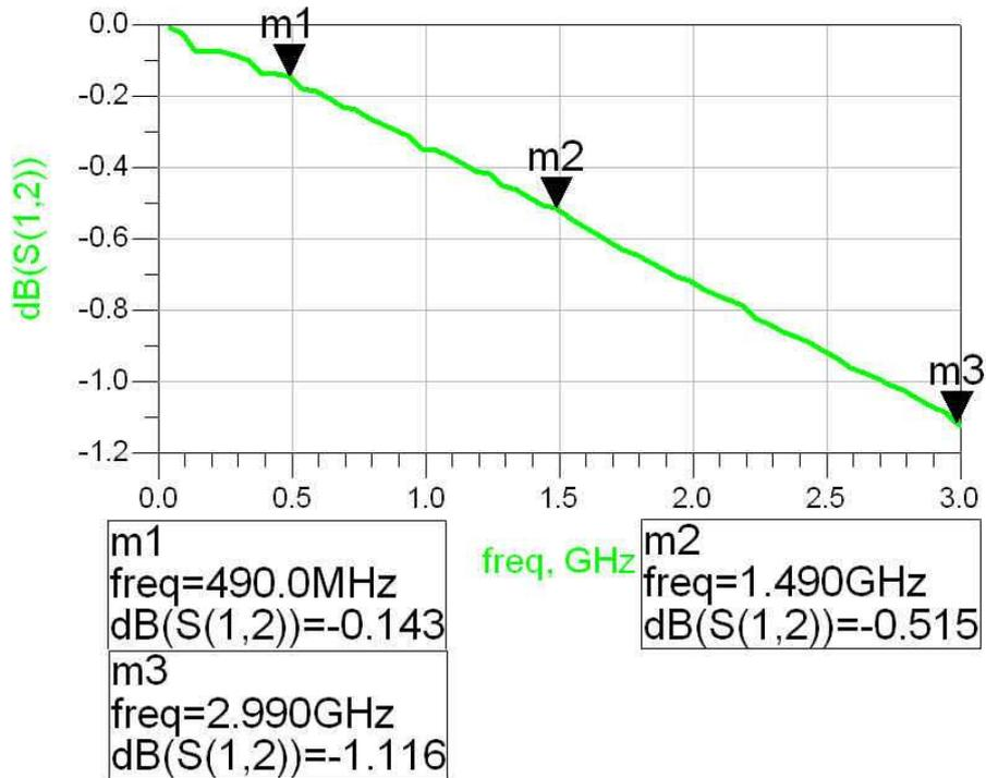
the measurement includes the insertion loss due to the test board and connectors
