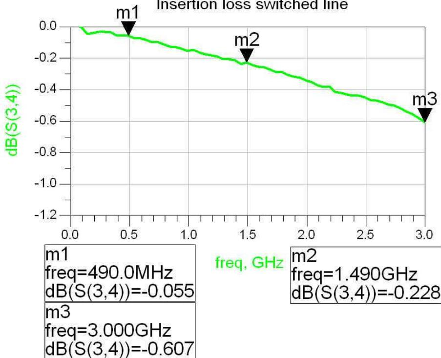
the measurement includes the insertion loss due to the test board and connectors
