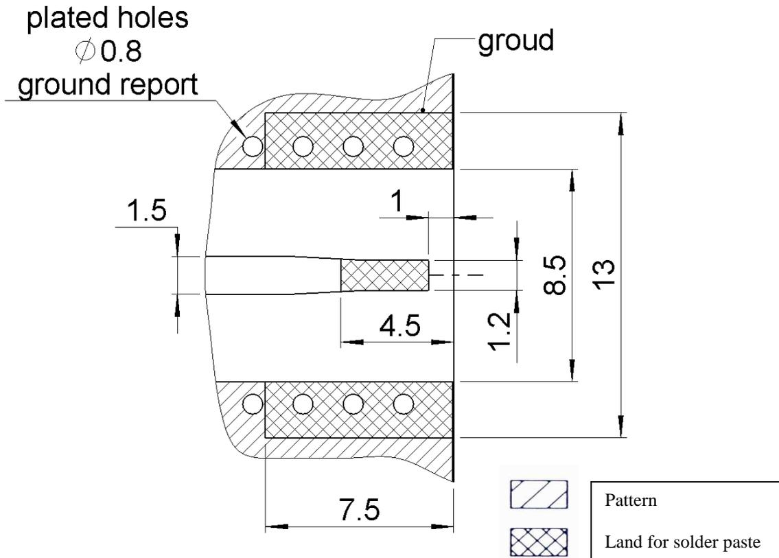
Thickness of PCB : .063 (1.6 mm)
