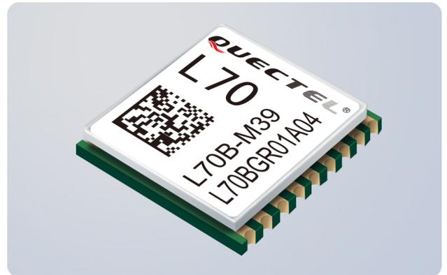
L70, an SMD type module, brings the high performance of MTK positioning engine to the industrial applications with compact profile, ultra low power consumption and fast positioning capability.
