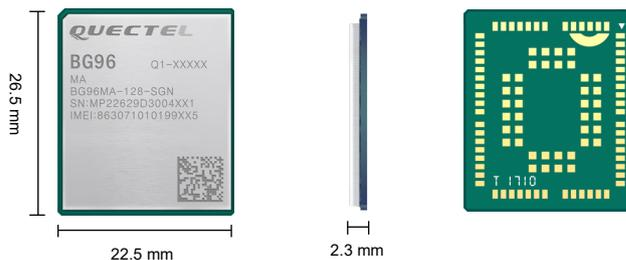
BG96 is an LTE Cat M1/Cat NB1/EGPRS module offering maximum data rates of 375 kbps downlink and uplink. It features global frequency bands, ultra-low power consumption, and is compatible with Quectel LTE Standard module EG91/EG95, LPWA module BC95-G/BG95, UMTS/HSPA module UG95/UG96 and GSM/GPRS module M95.
