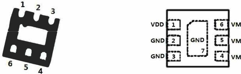
Figure 2. Pin Configuration
