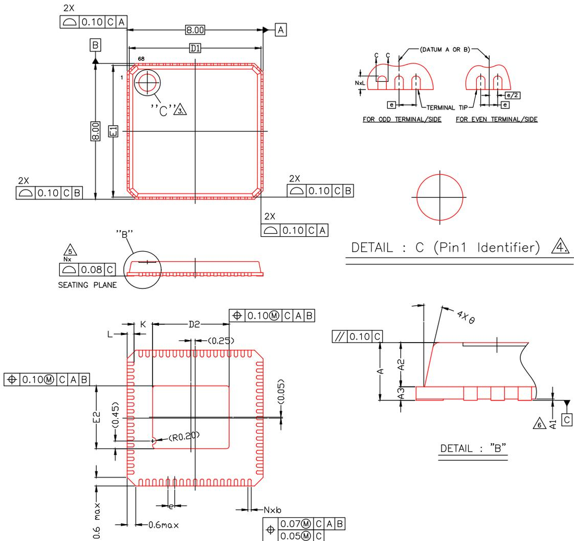
Figure 4-1 QCA4004 mechanical dimensions, top and bottom views
