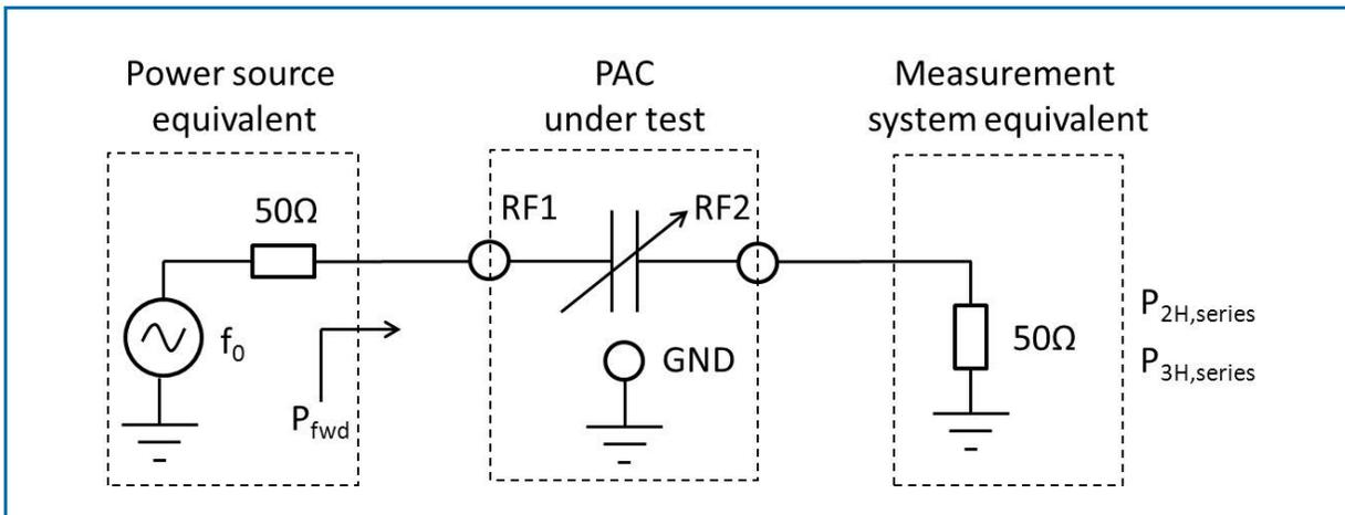
Series Configuration IMDs Measurement Set-up
