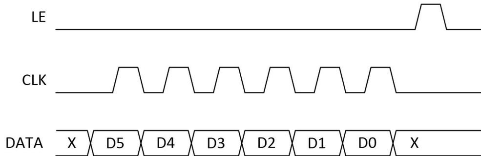
**Latched Parallel Mode Timing Diagram**
