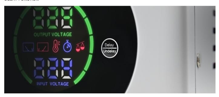
The stabilizer is equipped with a delay function. The default delay time is 6 seconds. This function is useful for products with motors and compressors to prevent and protect the device from damage due to frequent switching on of the device right after it is turned off. The maximum delay time is 180 seconds.
