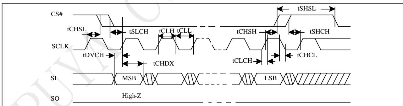
Figure 5-5 Output Timing
