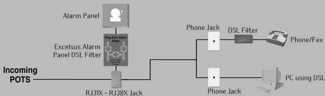
**Smart Protection for Your Customers - and Your Business** To keep DSL from interfering with alarm panel modems - and blocking alarm calls - just plug the panel's RJ plug into the Alarm Panel DSL filter. From then on, our patented technology ensures line seizure and cut-line protection, so alarm calls can go out. Install one on every job - to protect your customers who have DSL now, and to protect your customers who add it later.
