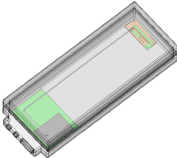
Position 2. Antenna could be mounted on upright position at bottom end of device
