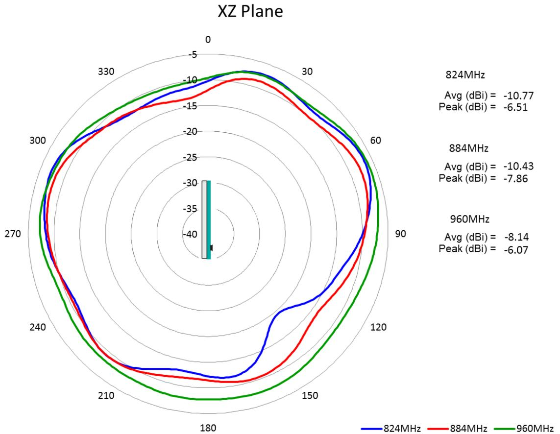
Note: Antenna tested on 2mm plastic plate with 200mm feed cable.
