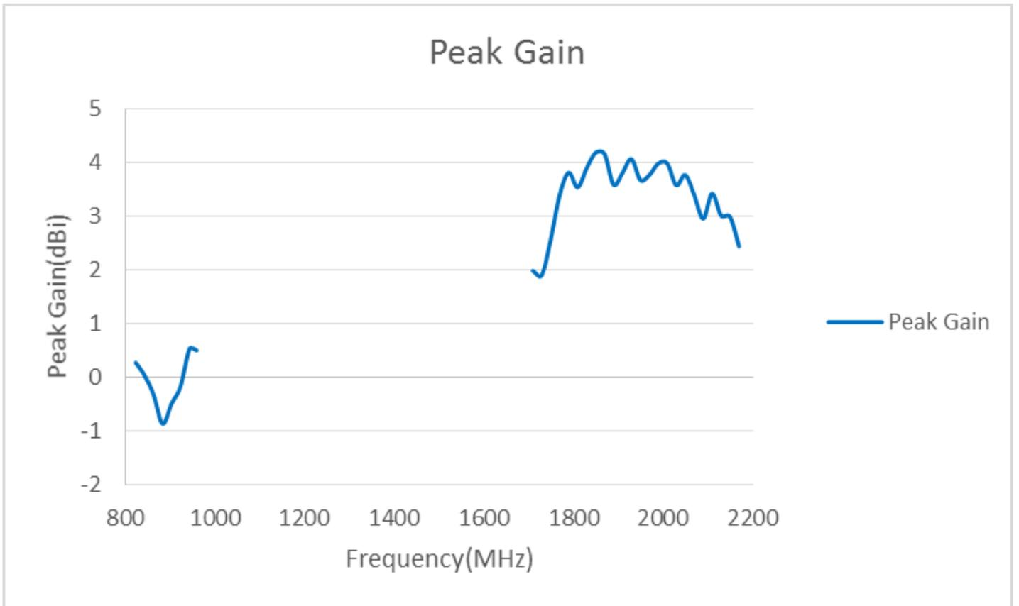
Note: Antenna tested on 2mm plastic plate with 200mm feed cable.
